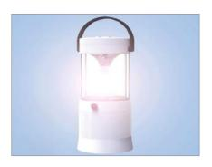
Salt water is all you need to power this Lamp for 80 hours. Hitachi Maxell's Mizusion lamp is equipped with a reservoir at the top that holds the salt water. A replaceable magnesium "power bar" interacts with the salt water and oxygen to produce the positive and negative electrons that generate the electricity. The lamp can provide up to 2000 lux of illumination, and can be used both indoors and out.
